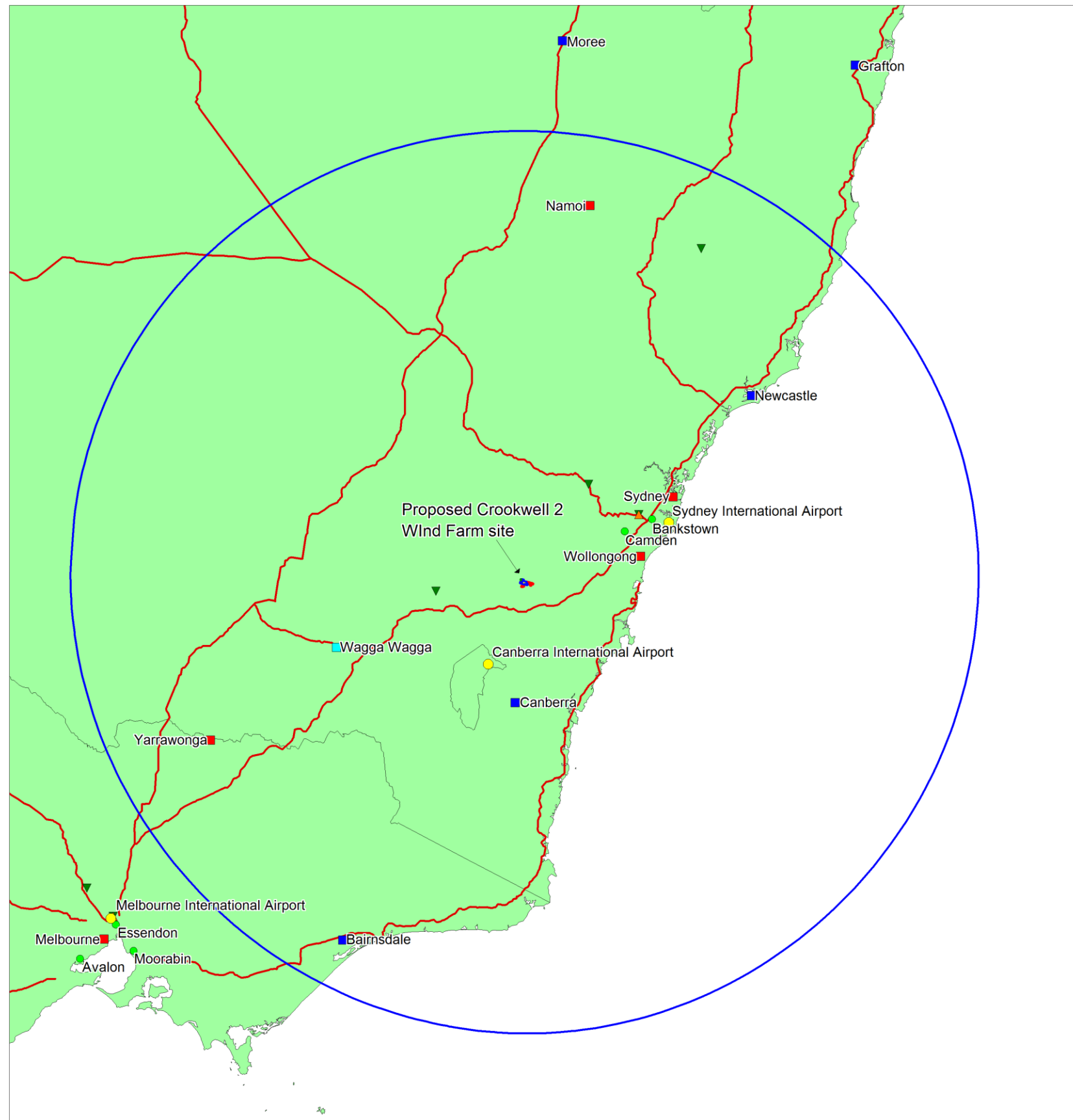
Figure 7 Location of major airports and meteorological radar sites within 250 nautical miles of the proposed Crookwell 2 Wind Farm
