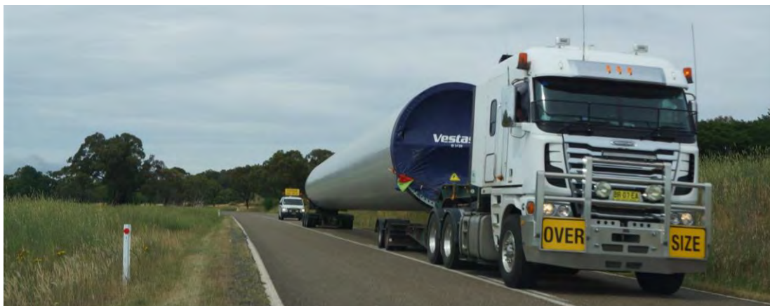
Figure 2.4: Typical Oversize Load (Tower Section)
